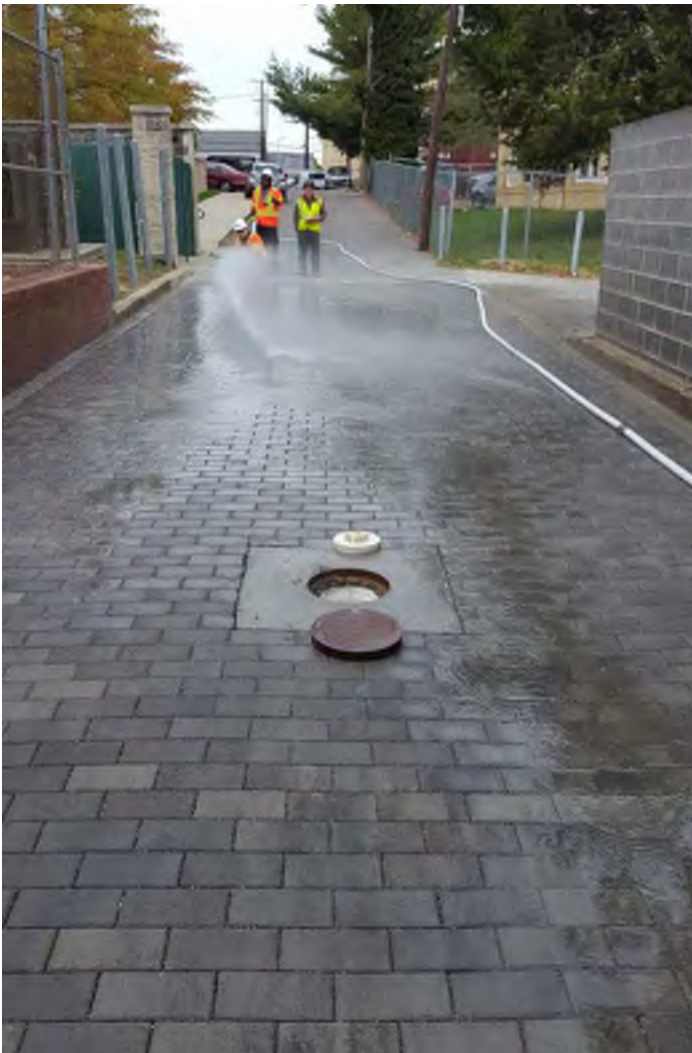
Crew performing hydraulic testing on a permeable pavement surface.
