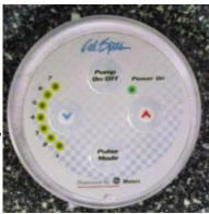
pump must be on prior to operating any other features of this system.
