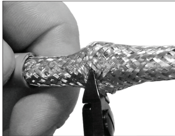
Figure 33 Cable Braid Bulge/Cutting
