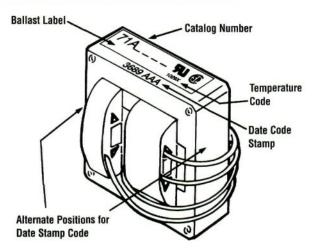
ADVANCE <sup>©</sup> HID Core & Coil ballasts are date stamped on either the top surface or the side surface of the ballast core. The four-digit number represents the *week* and *year* of manufacture. The first two numbers indicate the week and the last two indicate the year the ballast was manufactured. The example shows a ballast manufactured during the 36th week of 1989. The three letters are an Advance factory code.
