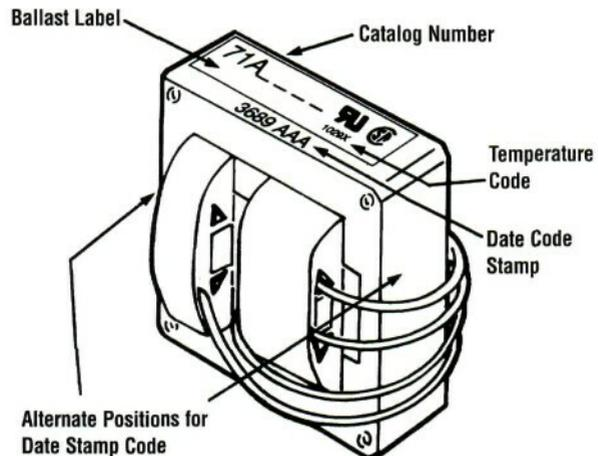
ADVANCE® HID Core & Coil ballasts are date stamped on either the top surface or the side surface of the ballast core. The four-digit number represents the *week* and *year* of manufacture. The first two numbers indicate the week and the last two indicate the year the ballast was manufactured. The example shows a ballast manufactured during the 36th week of 1989. The three letters are an Advance factory code.
