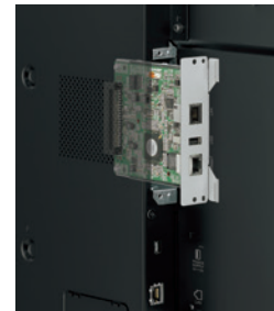
An optional board can slide into the slot on the back of the monitor.
