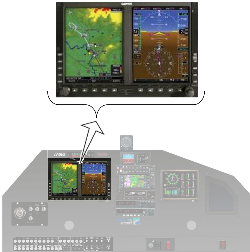
Figure 7-14 Instrument panel with optional GDU620 (MFD/PFD) unit (Optional configuration applicable to all aircraft)
