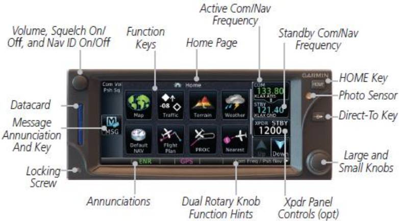
Figure 7-40 GTN650 NAV/COM/GPS unit description
