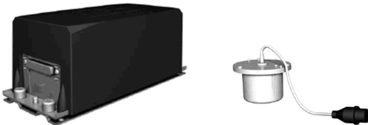
Figure 7-24 GRS77 AHRS - GMU44 Magnetometer
