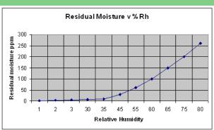
Water content of oil increases as it is exposed to high relative humidity
