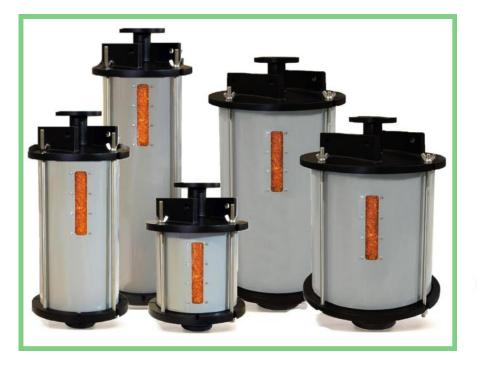
These Transformer Breathers are connected either by a flange or pipe thread connection. Mounting brackets on the top plate provide additional support for the Transformer Breather. Two-way, low pressure valves are fitted in the base plate of the breather to ensure that the atmospheric air enters the desiccant when a negative pressure differential occurs within the Transformer being protected.
