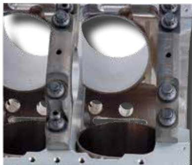
BILLET MAIN CAPS INSTALLED WITH SPLAYED BOLT PATTERN
