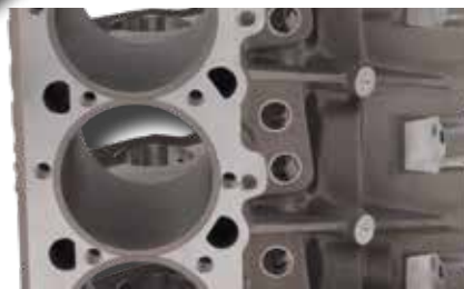
SLEEVES WITH THICK REGISTERS INSTALLED ASSURING PROPER RING SEAL
