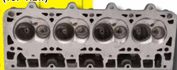
BR 7 - MACHINED FOR CROWER (TOP VIEW)
