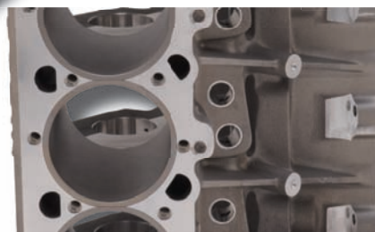
SLEEVES WITH THICK REGISTERS INSTALLED ASSURING PROPER RING SEAL
