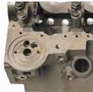
OIL FILTER MOUNTING BOSS IS DESIGNED FOR BOLT-ON OIL FILTER ADAPTER
