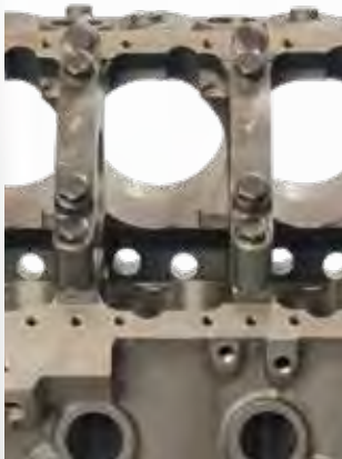
NODULAR IRON 4-BOLT SPLAYED MAIN CAPS
