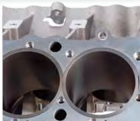
SLEEVES WITH THICK REGISTERS INSTALLED ASSURING PROPER RING SEAL
