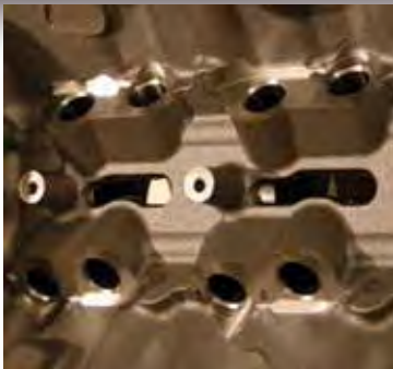
LIFTER BORES AVAILABLE: .842 OR .903 BORE DIAMETER
