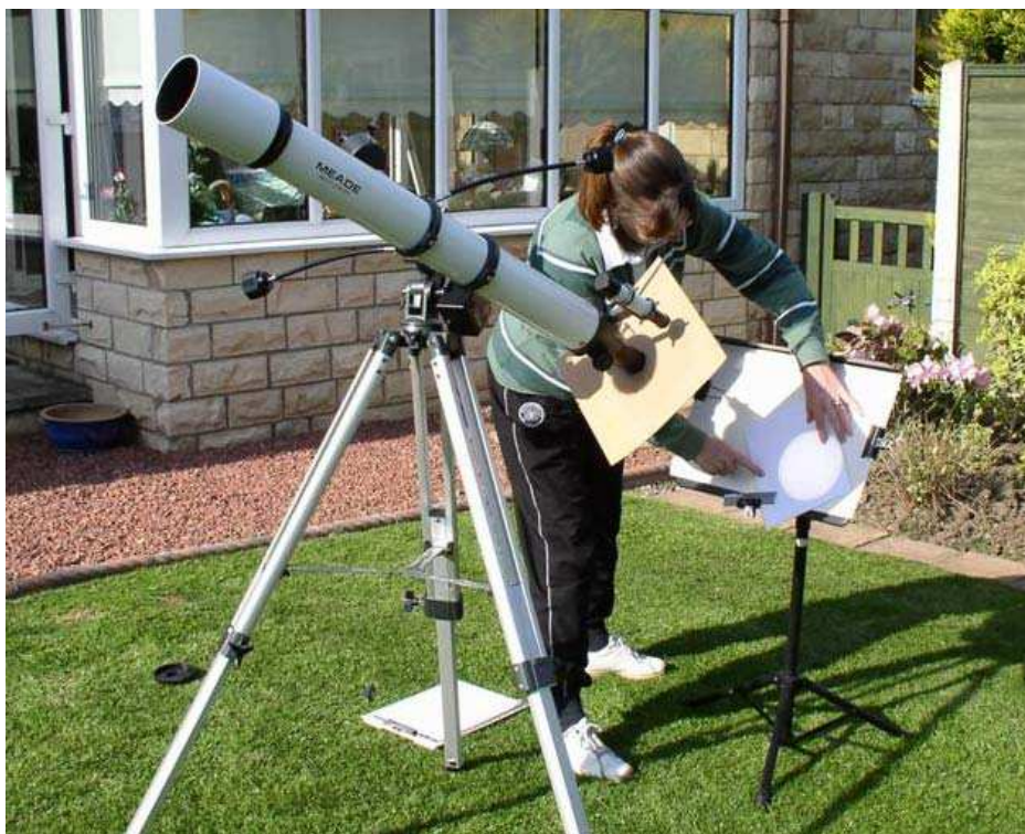
Projecting an image of the Sun with a small refractor.
