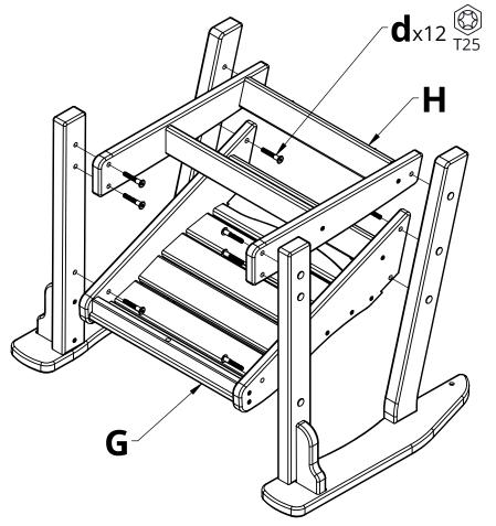
**4.** Attach Parts H & I to the previous assemblies using Hardware d, this step is made easier if performed with the assembly upside down
