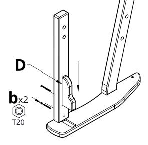
**2.** Attach Part D to the previous assemblies using Hardware b
