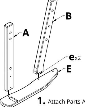
1. Attach Parts A & B to Part E by inserting Hardware e into the predrilled holes and rotating Parts A & B clockwise, stopping when the assembly is tight
