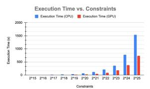
Figure 3: Groth16 CPU and GPU (A10) performance on proof generation as a function of number of constraints.
