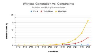
Figure 8: Comparing the PlonK family in performance on the witness-generation component of ZK-proof generation.
