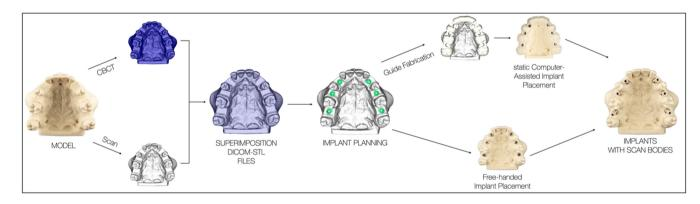
FIGURE 2 Visual depiction of the methodology followed for the static Computer-Assisted Implant Placement group.
