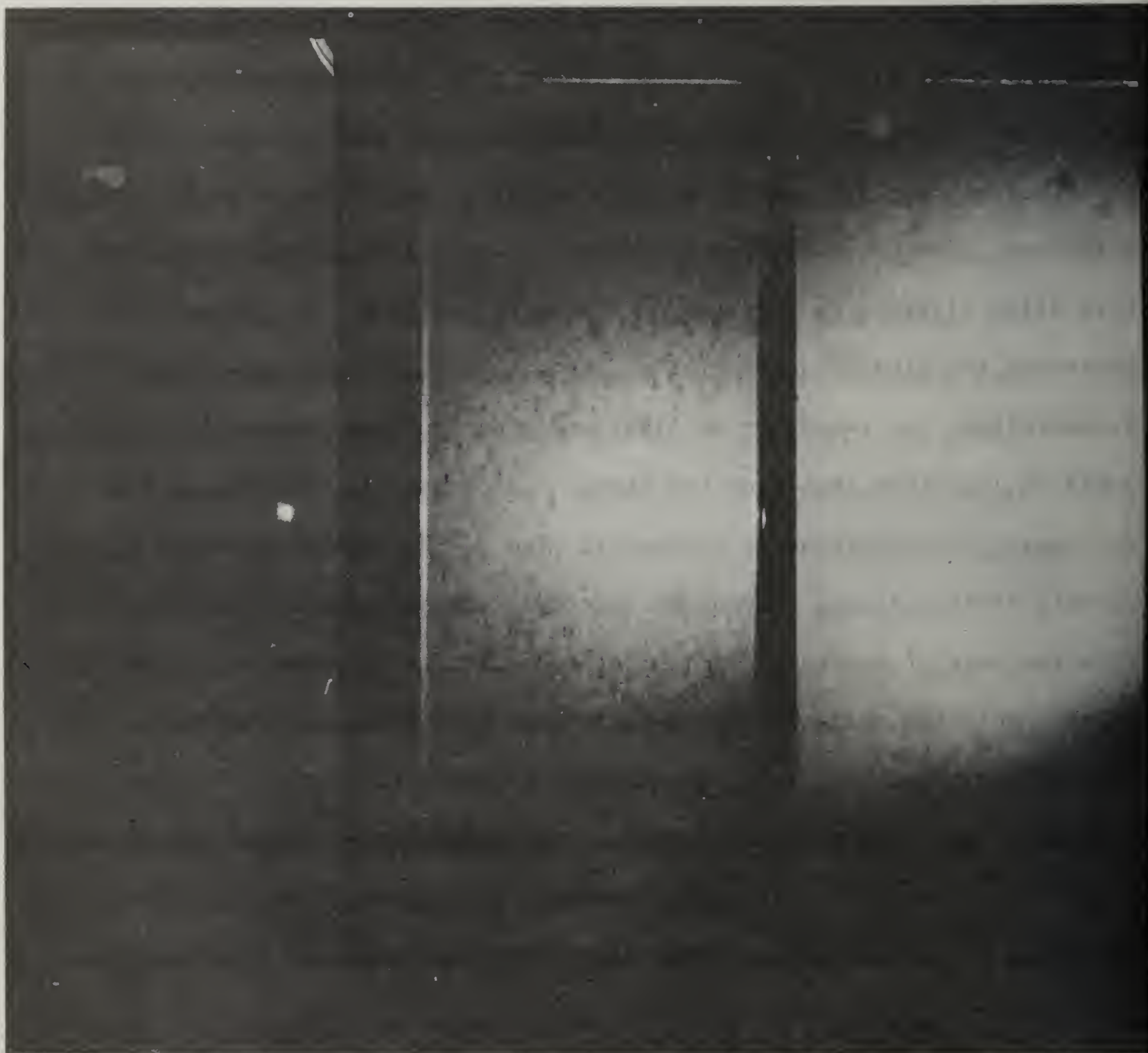
Fig. V-5 POINT SOURCE OF LIGHT VIEWED THROUGH GLASS PLATES HAVING VARYING DEGREES OF TRANSLUCENCY
