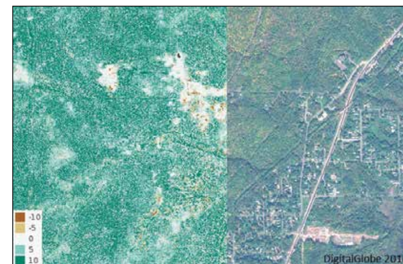
Figure 2: Duluth, Minn. On the left is a digital surface model difference map, using a LiDAR-derived surface model acquired in Spring 2011 and submeter stereo imagery-derived surface model from Fall 2016. The optical image on the right is from the same acquisition as the digital surface model in Fall 2016. Imagery courtesy of DigitalGlobe and the NextView program.
