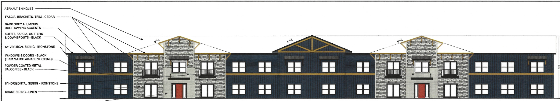
FRONT ELEVATION - 2 STORY DARK SCHEME SCALE: 1/8" = 1'-0"
