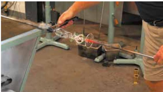
15) The goblet is transferred to a pontil (or 'pundy'), a metal rod with a small amount of molten glass on its hot end; this acts as a handle for the conclusion of the manufacturing process. The constriction near the blowpipe (see fig. 2 above) is broken.
