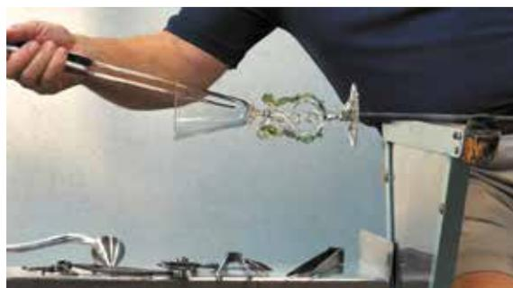
16) After reheating the uppermost part of the cup, the jacks and soffietta (a conical metal inflating-tool) are used to give the cup its final form.
