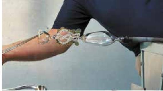
14) A hole is made in the end of the bubble, and after reheating the glass the jacks are used to create a folded edge and then give the foot its final shape.
