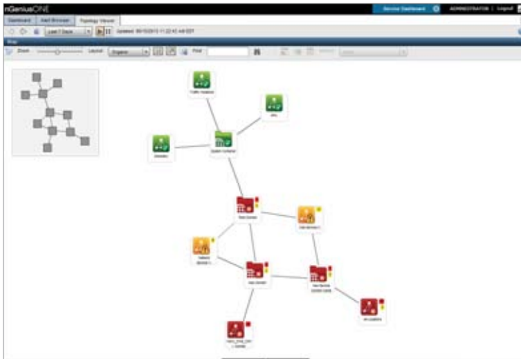
Figure 4: The nGeniusONE Service Dashboard topology map feature illustrates server and application interrelationships within a service domain.
