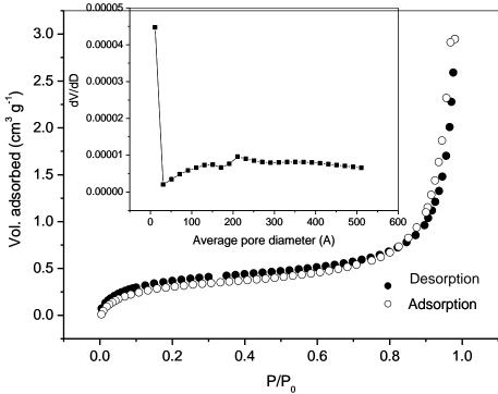
Fig. 6. Nitrogen adsorption and desorption isotherms and distribution of pore diameter (inserted figure)
