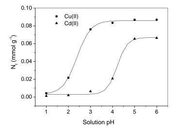
Fig. 7. Effect of solution pH on adsorption of Cu(II) and Cd(II) in aqueous medium
