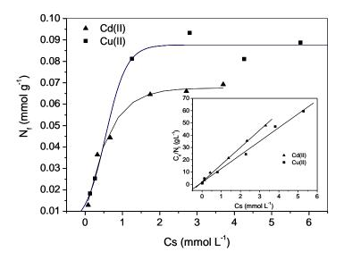
**Fig. 8.** Adsorption isotherms for Cu(II) and Cd(II) in aqueous solution at room temperature (28 °C) and linear shape of adsorption isotherms of Cu(II) and Cd(II) (inset)
