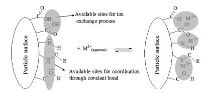
Fig. 3. Scheme of metal interaction with organic groups existing on the material surface during the adsorption process
