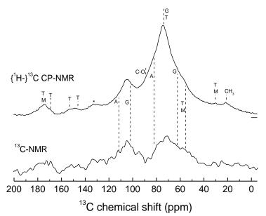
**Fig. 2.** <sup>13</sup>C NMR spectra obtained through {<sup>1</sup>H}-<sup>13</sup>C cross-polarization technique (upper trace) and with direct polarization of <sup>13</sup>C (lower trace). Code for resonance identification: T= thiamine, M= methionine, G= glucoside, A= apiosyl.
