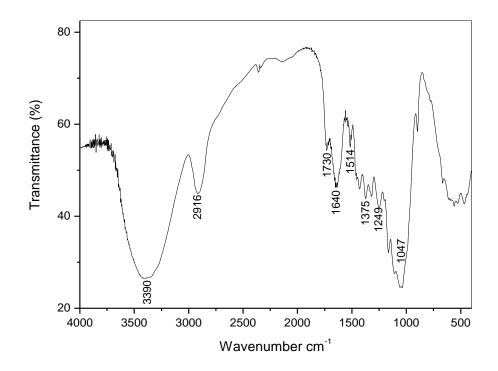
**Fig. 1.** Infrared spectrum of corn leaf powder with some organic group absorption bands; measuring conditions: 200 scans; resolution 4 cm<sup>-1</sup>; room temperature (28 °C)
