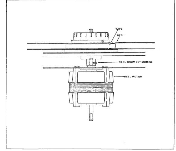
Figure 5-27. Reel Height Adjustment
