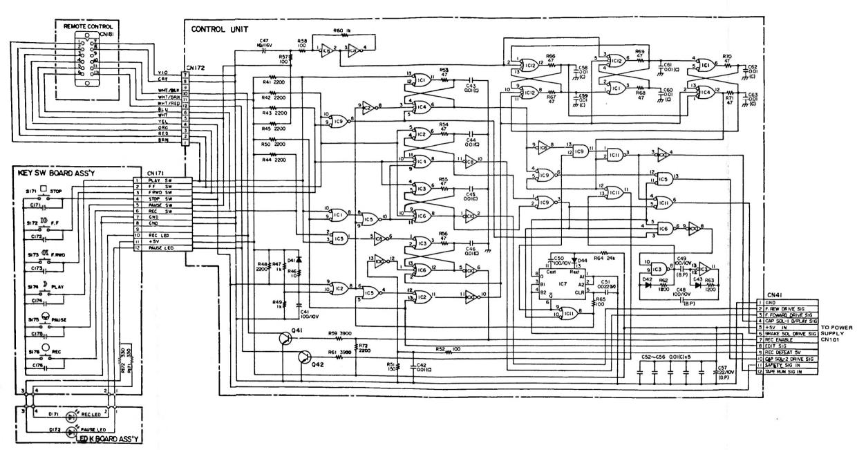
Figure 4-1. Control Unit Schematic
