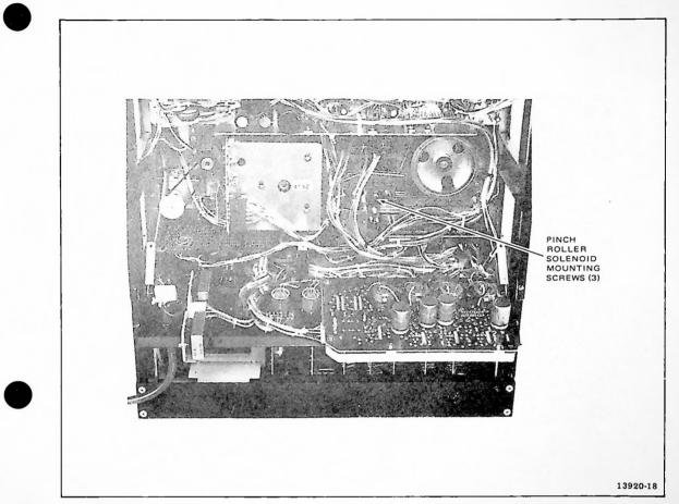
Figure 5-9. Pinch Roller Solenoid Mounting Screws Location
