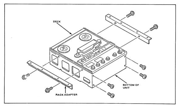
Figure 2-3. Rack Adapter Installation
