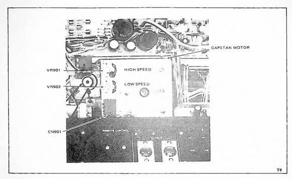
Figure 5-19. Tape Speed Adjustments
