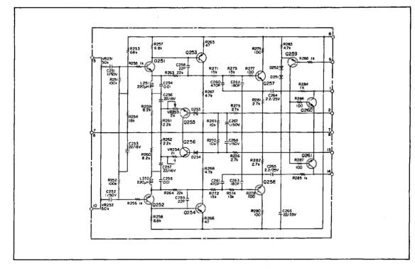
Figure 4-8. Reproduce Line Amplifier Schematic
