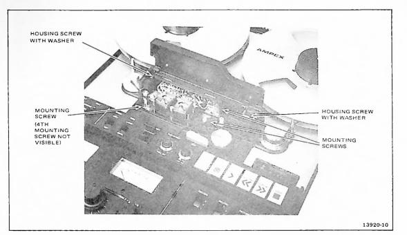
Figure 5-22. Head Assembly Removal
