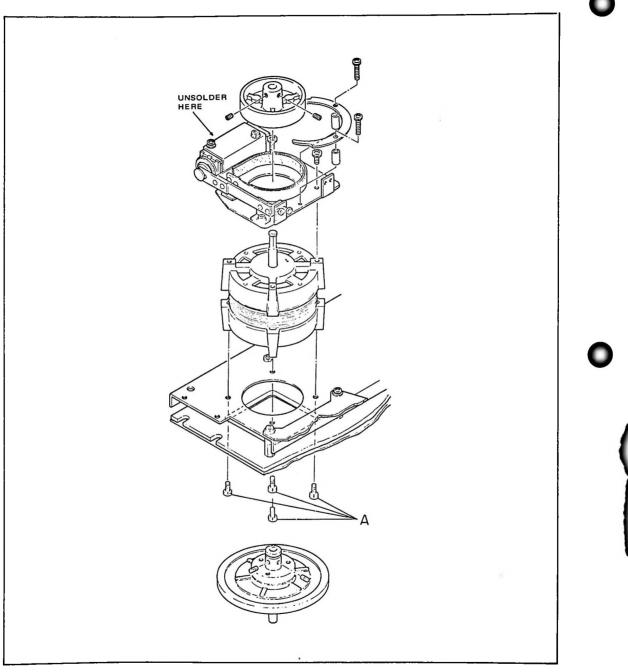
Figure 5-28. Reel Motor Assembly Removal
