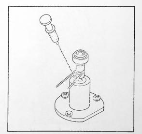
Figure 5-3. Digital Counter Roller Lubrication
