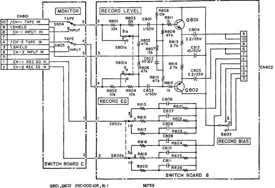
I ALL CAPACITOR VALUES ARE IN MICROFARADS, 50V 2 ALL RESISTOR VALUES ARE IN OHMS, 1/4 WATT, 5%
