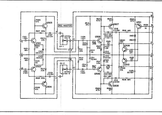
Figure 4-12. Mix Line Amplifier Schematic
