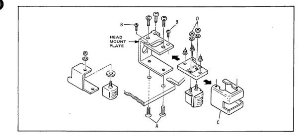
Figure 5-24. Head Disassembly
