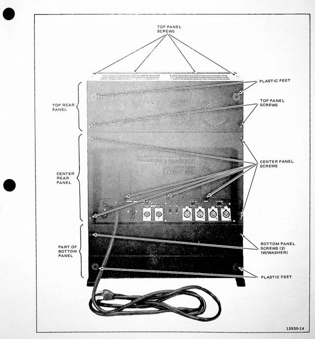
Figure 2-4. Screw Locations for Panel Removal
