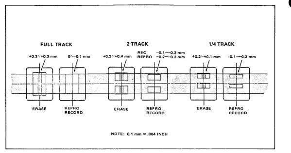
Figure 5-7. Tape Positioning for Head Alignment
