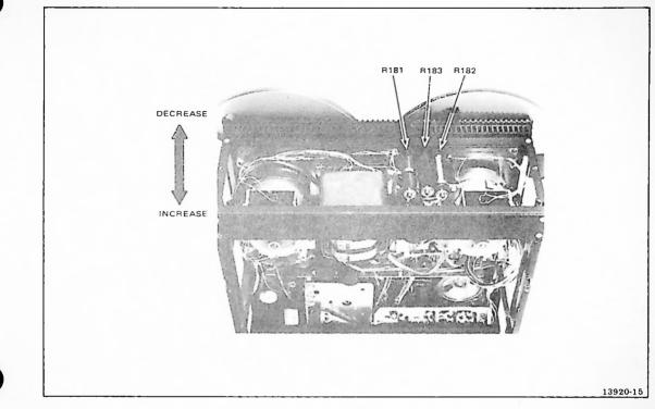
Figure 5-13. Tension Adjustment Resistors
