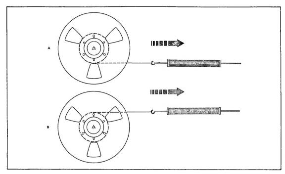
Figure 5-14. Brake Torque Measurement
