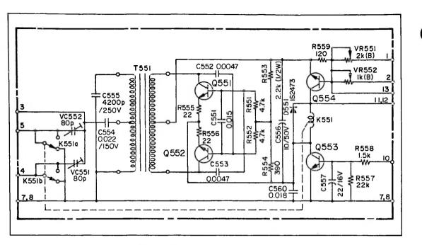
Figure 4-14. Bias Oscillator Schematic
