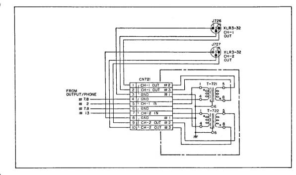
Figure 4-10. Output Transformer PWA Schematic
