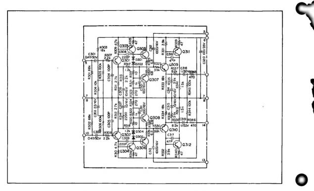
Figure 4-9. Output/Phone Amplifier Schematic
