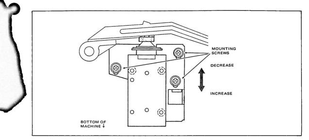
Figure 5-11. Pinch Roller Pressure Adjustment
