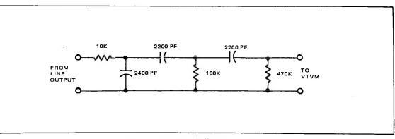
Figure 5-16. ASA "A" Weighted Filter
