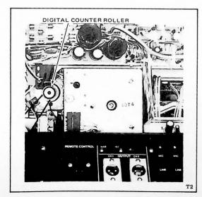
Figure 5-2. Digital Counter Roller Location
