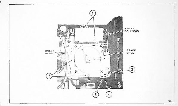
Figure 5-15. Brake Assembly
