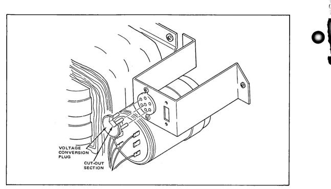
Figure 2-6. Voltage Conversion Plug
