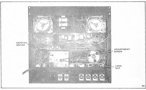
Figure 5-5. Capstan Shaft Tolerance Adjustment
