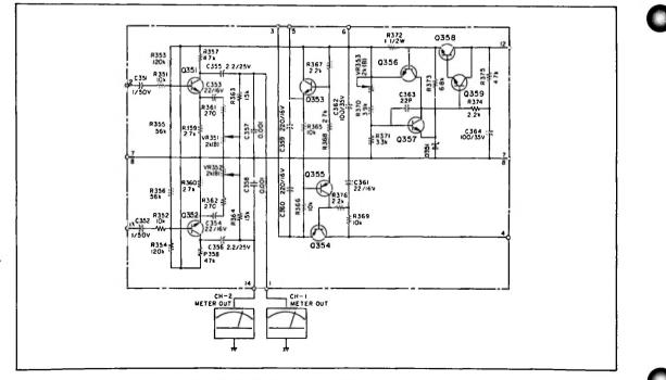
Figure 4-15. Meter Amplifier/Stabilizer Schematic
