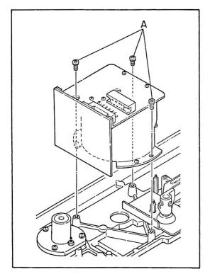
Figure 5-25. Capstan Motor Removal
