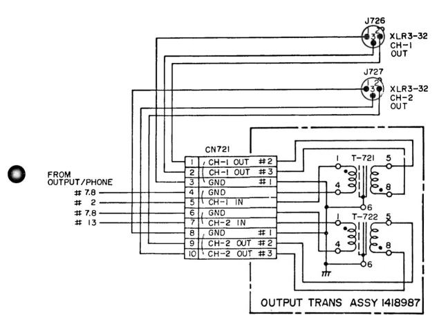
Schematic No. 1418961. Output Transformer PWA
