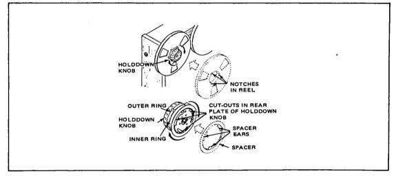
Figure 3-2. Large Hub Reel Installation
