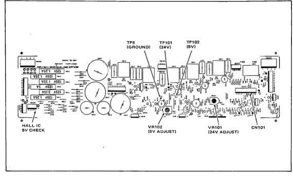
Figure 5-18. DC Voltage Adjustment, Power Supply PWA
