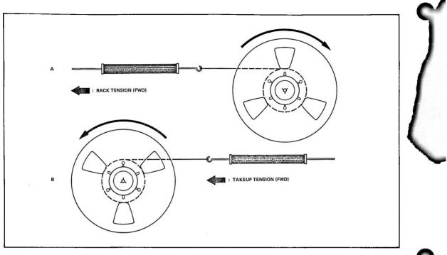
Figure 5-12. Tension Measurement
