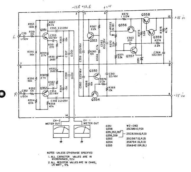
Schematic No. 1418971. Meter Amplifier/Stabilizer
