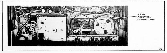
Figure 5-23. Head Assembly Connectors
