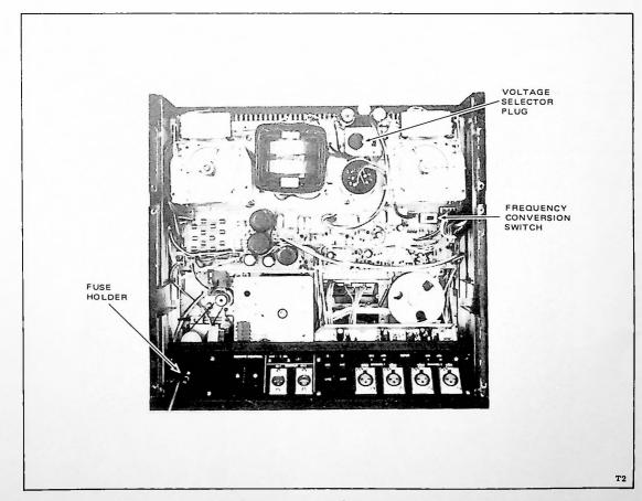
Figure 2-5. Voltage and Frequency Conversion
