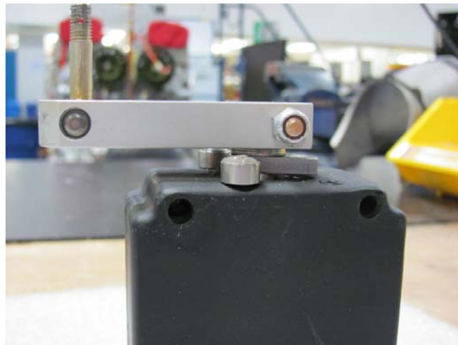
Figure 2. Magnetic brake assembly with stops properly installed.
