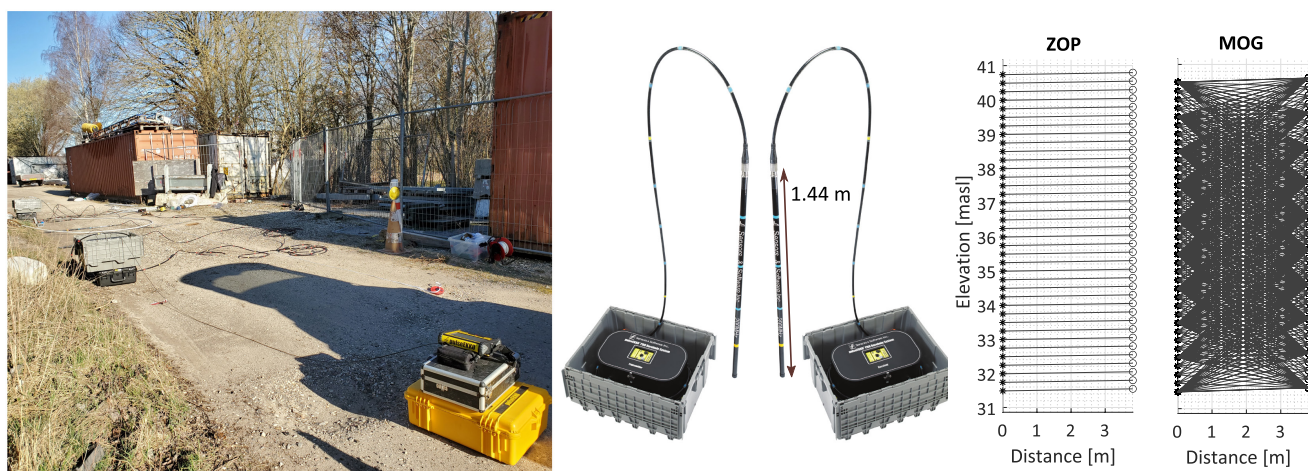
Figure 2. Left: Photo of the field site with the GPR equipment. Antennas are laid out on ground during warm up of the equipment. Middle: Schematic illustration of GPR transmitter and receiver boxes connected to the 100 MHz antenna https://www.sensoft.ca/products/pulseekkopro/borehole-gpr/ (with permission from Sensors&Software). Right: Data acquisition geometry of ZOP data and MOG data. Asterisks indicate transmitter positions and circles indicate receiver positions. The lines indicate the straight wave paths for the propagating EM signal between a given transmitter and receiver position.
