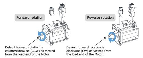
The rotation direction of the Motor can be changed by setting the Motor Direction from the Basic Setup page in the drive commissioning screens. The figure above shows the default setting.
