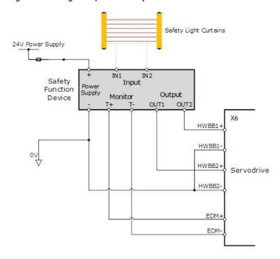
Use armored cables to protect the HWBB1+ and HWBB2+ from short circuits. Use the EDM signal at the common emitter output, making sure that the current flows from EDM+ to EDM-.
