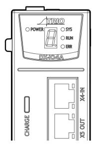
The POWER LED indicates power is present to the Control board.
