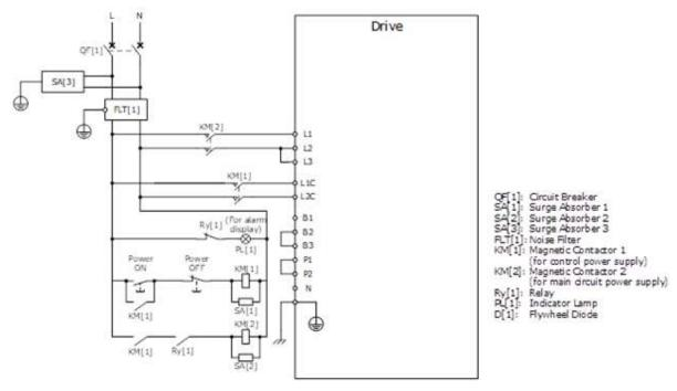
NOTE: for single phase wiring L or N can be wired into either L1 or L2
