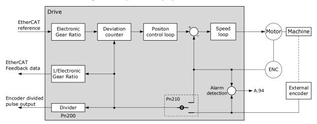
This setup can be useful in some high-precision positioning applications where there is compliance or backlash between the motor and the load.
