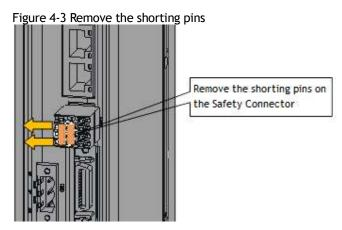
Step 2 Wiring the Safety Function Device
