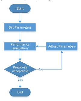
There are various indicators used to evaluate servo performance including bandwidth, response time, overshoot, steady state error, anti-load disturbance, speed ripple fluctuation, torque ripple, etc. The importance of these will depending on the application.
