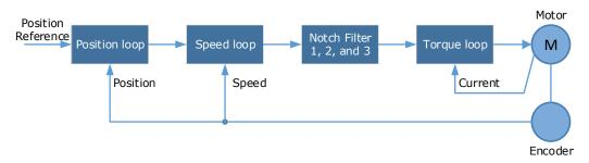
The diagram below shows the relevant parameters for the notch filter.
