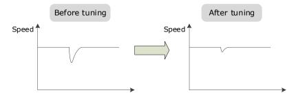
Tuning the load torque compensation function can be used to improve the anti-load disturbance performance, considering that the reference response performance and the load disturbance resistance cannot be balanced.
