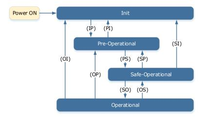
Figure 9-1 EtherCAT state machine
