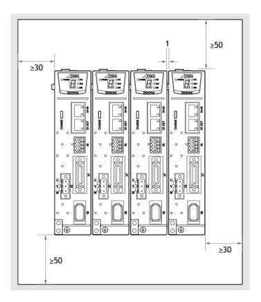
The DX4 can be mounted so that the distance between adjacent Drives is 1mm.
