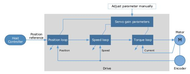
It is necessary to adjust the three-loop control parameters of the Servo from the inside out, that is, the adjustment sequence is  $\boxed{\text{Torque loop}} \rightarrow \boxed{\text{Speed loop}} \rightarrow \boxed{\text{Position loop}}$ . In order to maintain stability, the bandwidth setting should be the largest in the torque loop, then the speed loop, and the position loop should be smallest.
