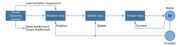
This function is based on the Model Following Control (7.6) and enabled via Pn150.
