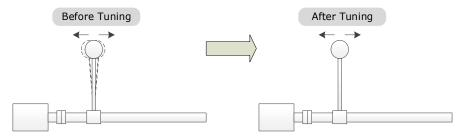
The aim of the Model Following Control is to maintain the stability of the load position based on a relationship between load position and Motor position. This is done by correcting the position reference and generating new speed and torque feedforward values.
