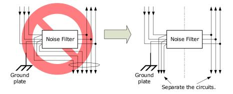
• Separate the Noise Filter ground wire from the output lines. Do not place the Noise Filter ground wire, output lines, and other signal lines in the same duct or bundle them together.
