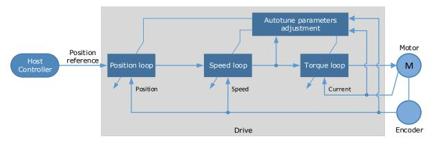
When using the tuning-less function, the following parameters are automatically adjusted.
