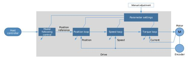
The Model Following Control function is enabled via Pn150.
