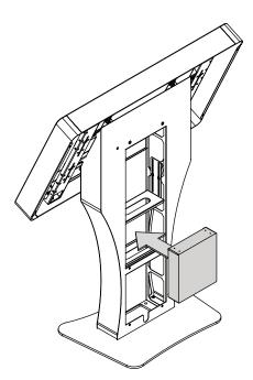
9-3 New cover bracket so it rests on media player. Tighten crews to secure bracket in place.
