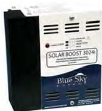
The **SB3024iL** is designed to charge 12 and 24 DC battery systems from a 24 VDC array (maximum open-circuit voltage is 57 VDC). Maximum charge current is 40 A output at 12 VDC and 30 A at 24 VDC. It has an auxiliary output that can serve as a 20 A load controller or as a 2 A battery charger. The **SB3024DiL** version adds a front-mounted digital display which shows battery voltage, solar current, charge current, and charge mode. A second display can be used as a remote display up to 300' away,
