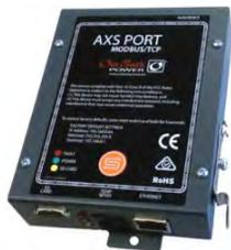
The SunSpec-compliant **AXS** Port Modbus/TCP Interface provides similar functionality to the MATE3, including access to OutBack Power’s OPTICS RE platform, but must be accessed via Ethernet. Custom user interfaces can be developed if an independent monitoring system is used. System data logs can be downloaded using Modbus-read or FTP transfer.
