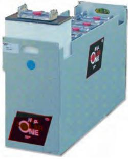
The Solar-One® battery with HuP® Technology is optimized for renewable energy systems. It has a slightly enlarged epoxy-coated steel case that allows cell removal so it can be installed by parts without a forklift or crane. Solar-One® batteries are designed with 0.310" thick positive plates and a patented technology that allows them to be rated for 4,000 cycles to 50% depth of discharge. The 10-year warranty, 7-year full replacement, and 3-year prorated, is the best in the industry.
