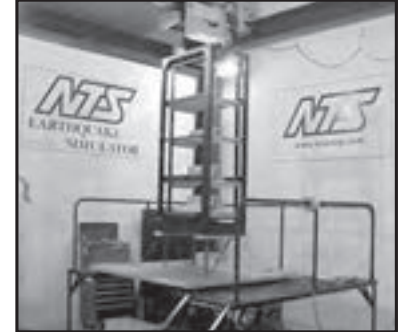
Seismic testing of the Raised Floor Kit. PART# AFSB18, cabinet sold separately
