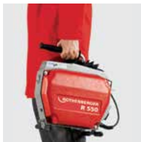
Drive lever locked in stop position — serves as carrying handle
