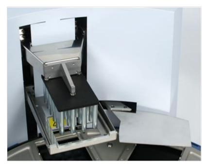
Figure 24. KingFisher Flex head for KingFisher 24 deep well plate fitted
