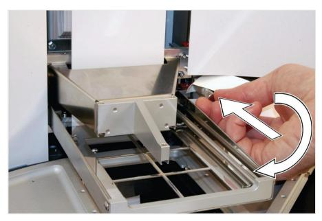
Figure 30. Fit the transport lock of the tip comb holder
