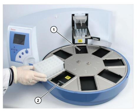
Figure 40. Combine the tip comb and KingFisher plate (B)
