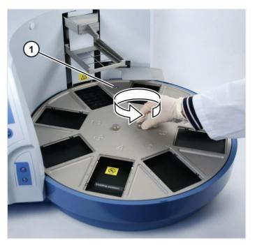
Figure 50. Unfasten the two finger screws
