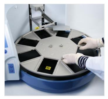
Figure 51. Remove the turntable
