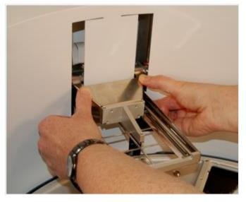
Figure 28. Press the tip comb holder downwards
