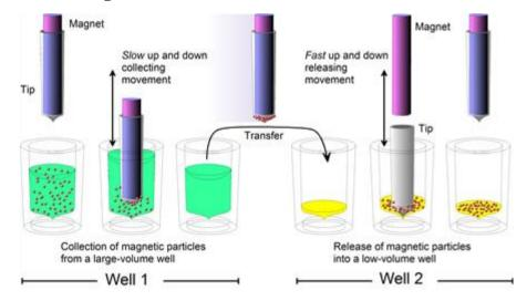
Figure 8. A concentration step during magnetic particle processing
