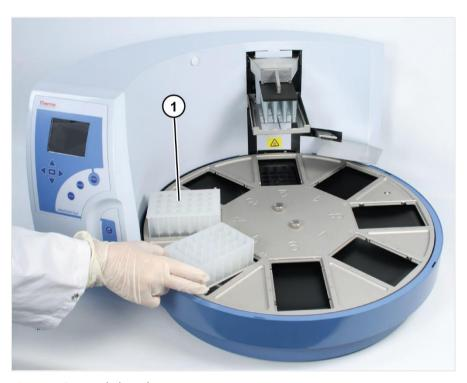
Figure 42. Load the plates
