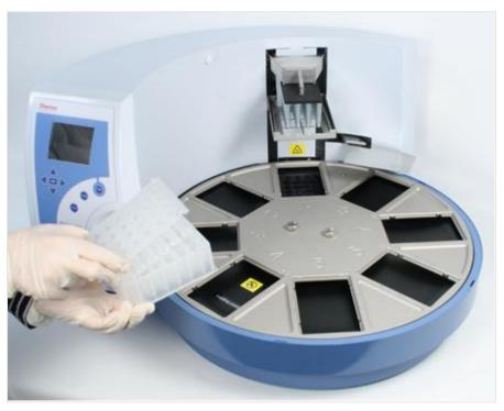
Figure 39. Combine the tip comb and KingFisher plate (A)
