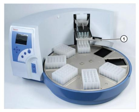
Figure 44. Tip comb in the tip comb holder
