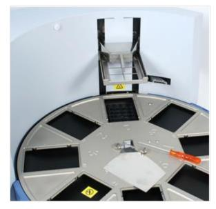
Figure 15. Shield plate prior to fitting
