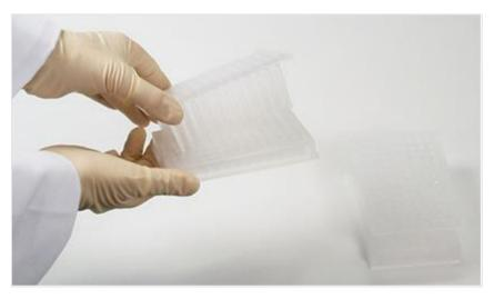
Figure 36. Store the other tip comb on a KingFisher 96 plate for further use
