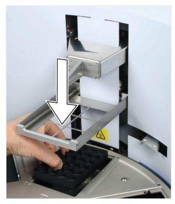
Figure 19. Insert the heating block
