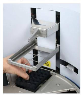
Figure 47. Insert the heating block
