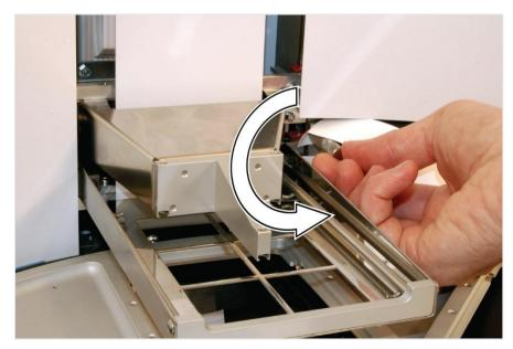
Figure 10. Remove the transport lock of the tip comb holder
