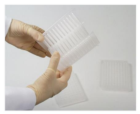
Figure 35. Separate the two tip combs
