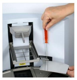
Figure 17. Fasten / loosen the shield plate
