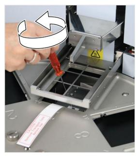
Figure 27. Refit the transport lock of the heating block (B)
