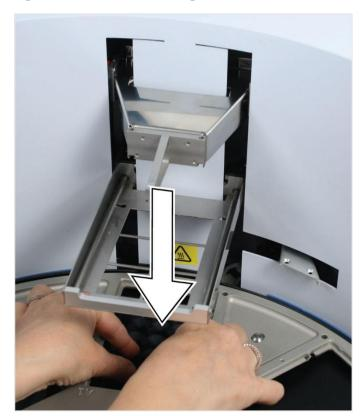
Figure 20. Press the heating block into place
