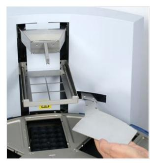
Figure 16. Insert the shield plate
