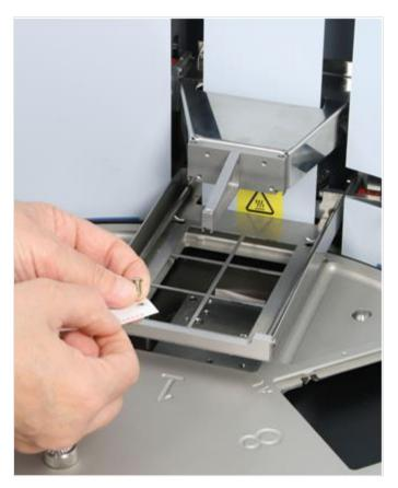
Figure 13. Remove the transport lock of the heating block (B)
