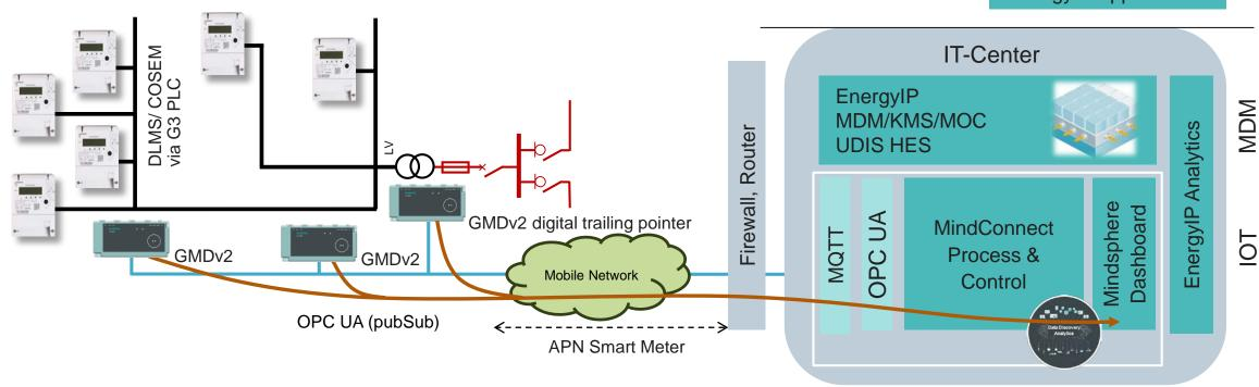
Determine system health precisely through analysis of voltage, reactive power, and outage data from available sensors and smart meters. Benefit from getting detailed and granular insights into momentary outages and reports.
