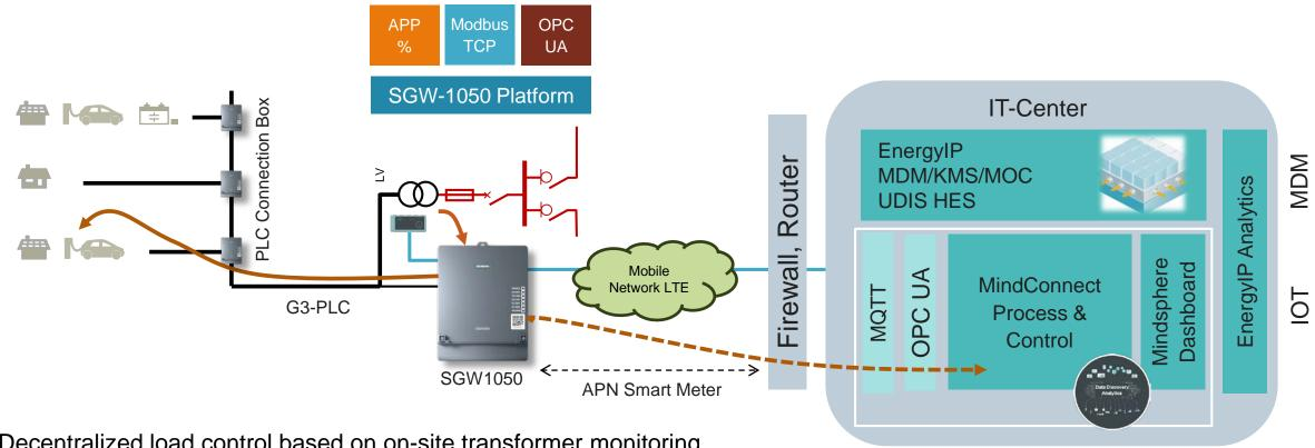
Decentralized load control based on on-site transformer monitoring...
