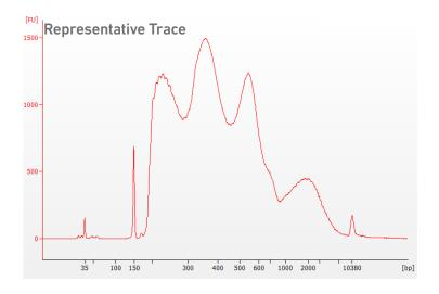
**b. OR** Run 2  $\mu$ l sample on the Agilent TapeStation High Sensitivity D1000 ScreenTape to determine fragment size.
