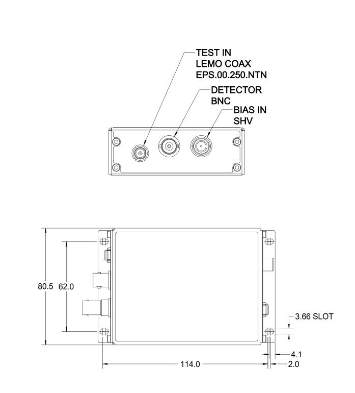
Figure 3. CR10 case (BNC signal connector option) end panel and plan view. Dimensions mm.
