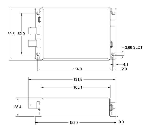
Figure 2. CR10 case plan and side views (SHV connectors). Dimensions mm.
