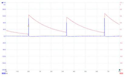
Figure 13. Injecting tail pulses to achieve a unipolar response to the test input
