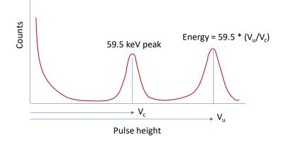
Figure 11. Determination of gamma energy by scaling
