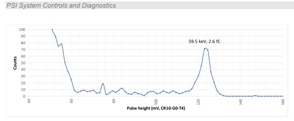
Figure 10. Measured pulse height spectrum for Am-241 gamma line, CR-110 and 1 µsec shaping
