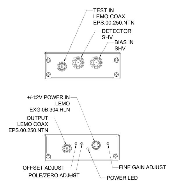
Figure 1. CR10 chassis end panels (SHV connectors). Dimensions mm.
