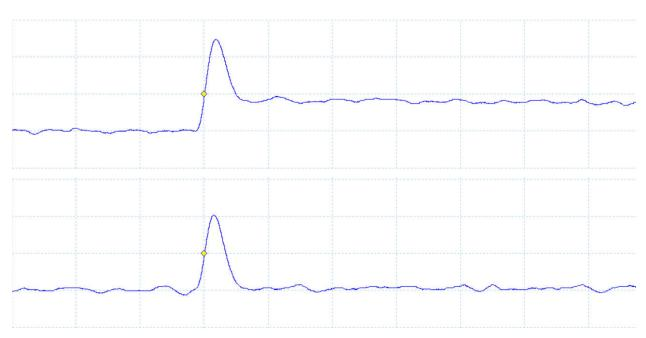
Figure 9. Incorrect pole-zero setting (top), correct pole-zero setting (bottom)
