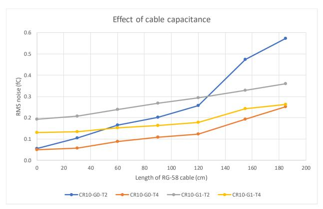
Figure 6. Effect of cable capacitive load on noise
