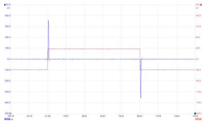
Figure 12. Effect of voltage square wave (red) injected into test input
