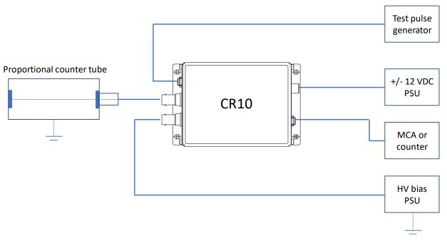
Figure 5. Schematic CR10 installation for readout of a proportional chamber
