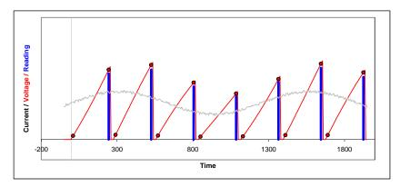
Figure 8 Repeated integrations to sample a continuous current signal.
