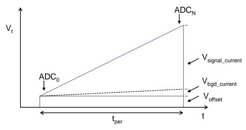
Figure 34. An integration showing signal and noise contributions to the final output.
