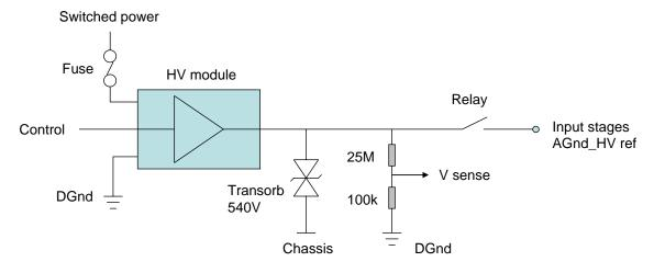
Figure 41. HV supply schematic for signal bias.
