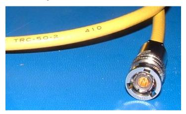
Figure 10. Triaxial cable with 3-lug triaxial connector
