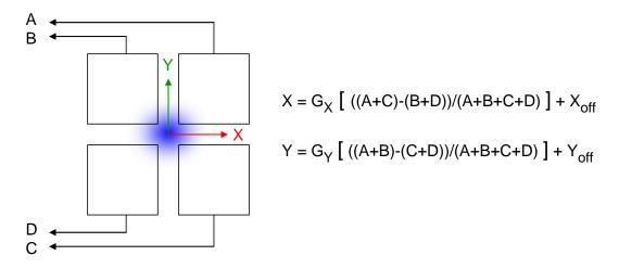
Figure 36. Two axis readout from a quadrant sensor
