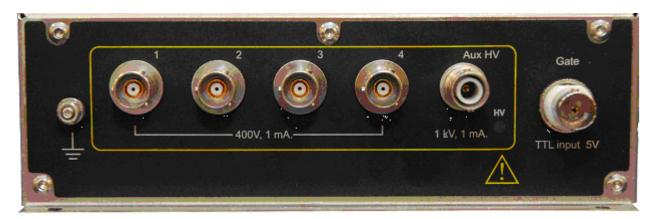
Figure 42. Front panel showing signal inputs, auxiliary HV output, gate input.
