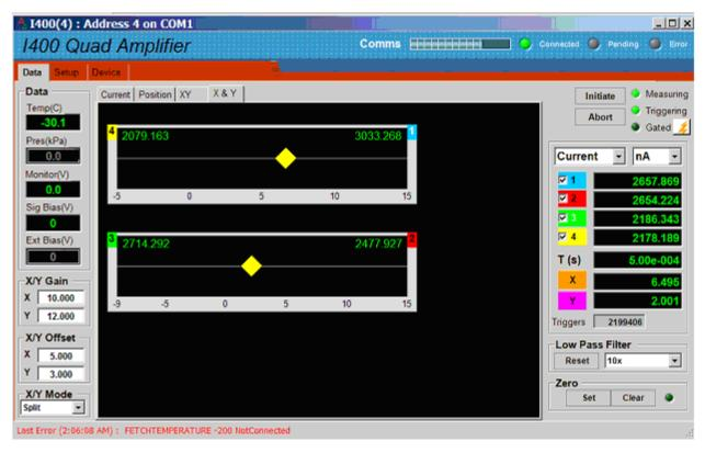
Figure 40. Independent X and Y position data tab, compensation factors, X/Y gains and offsets applied.
