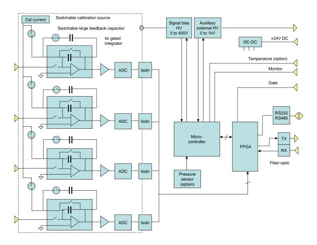
Figure 24. I400 block schematic.
