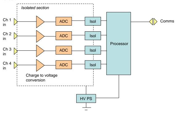
Figure 3. I400 block diagram.
