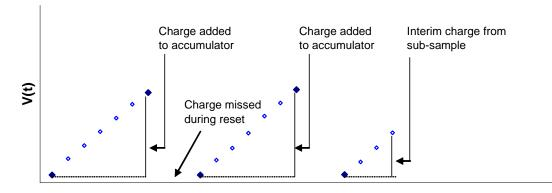
Figure 26. Illustration of integrator voltage at ADC sampling points during charge accumulation. The reset periods are shown relatively large.
