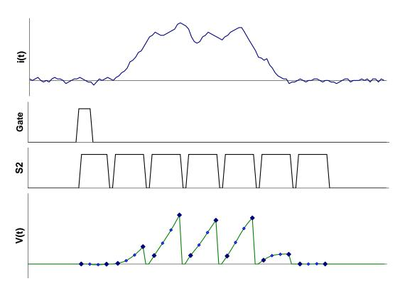
Figure 31. Example of an "external start" triggered measurement sequence started by a rising edge
