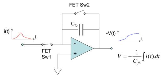
Figure 22. The basic gated integrator circuit.
