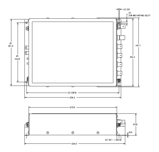
Figure 2. I400 case plan and side Dimensions mm.
