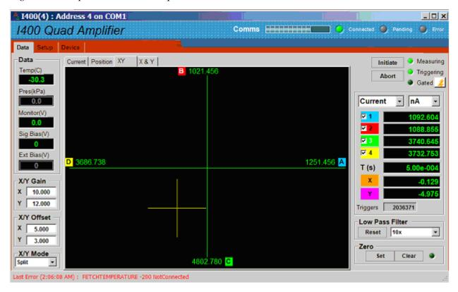
Figure 39. XY position data tab - split mode calculation
