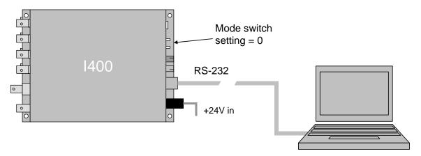
Figure 16. Direct RS-232 connection to the I400.
