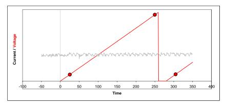
Figure 7. Discharging the integration capacitor and starting a new cycle.
