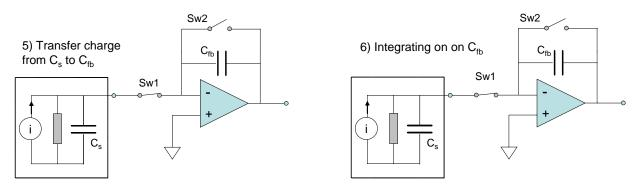
Figure 27. Switching sequence for the no-lost charge method.
