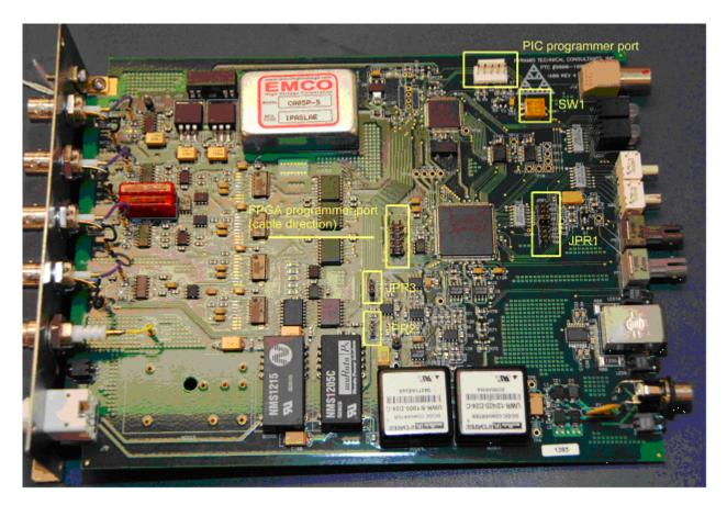
Figure 44. Internal switch and jumper locations.
