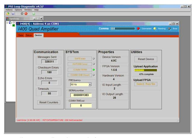
Figure 49. Microcontroller application upload in progress.
