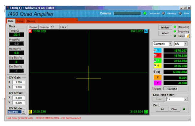
Figure 38. XY position data tab - quadrant calculation mode
