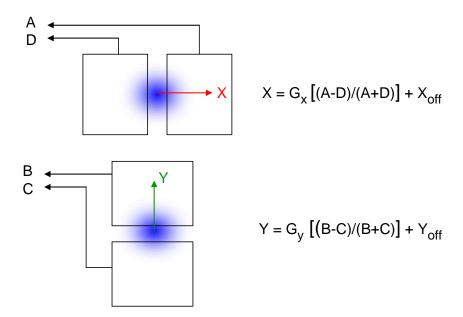
Figure 35. Split mode calculation. Signals A to D correspond to I400 channels 1 to 4.
