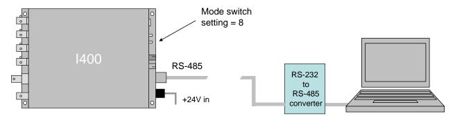
Figure 45. Using RS-485 as an RS-232 extender
