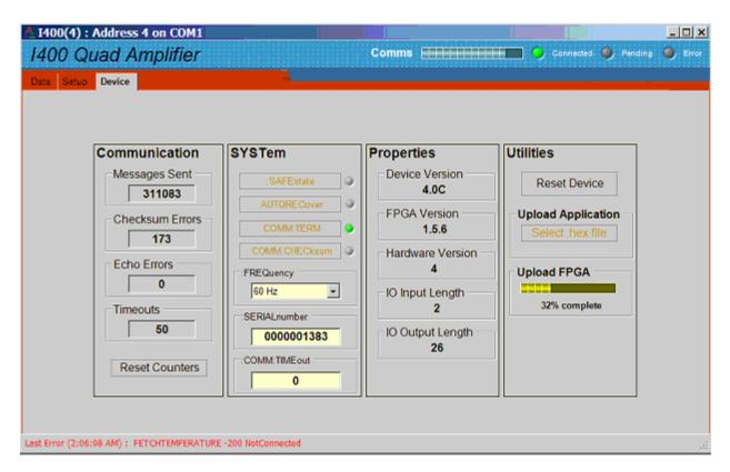
Figure 50. FPGA upload in progress.
