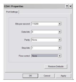
Figure 13. Hyperterminal COM port setup.
