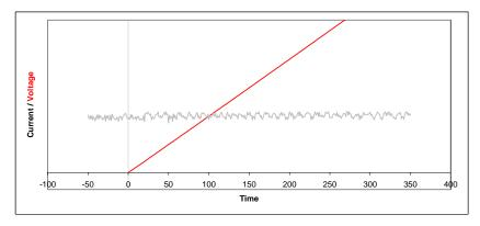
Figure 5. Voltage on a capacitor that is connected at time zero
