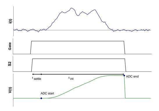
Figure 33. Illustration of a gated measurement.
