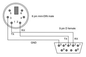
Figure 12. RS232 connection cable from the I400 to a PC serial port (DB9). Pins are shown looking at the face of the connectors.
