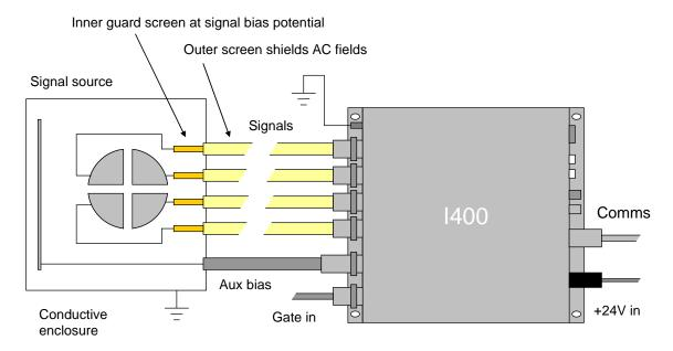
Figure 9. Schematic I400 installation
