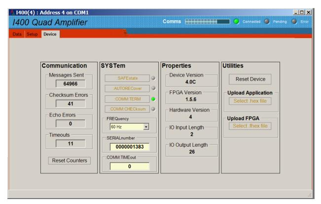
Figure 21. Device tab, showing firmware update utility controls.
