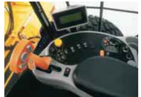
The floating operator console moves along with the seat to keep you comfortably in control at all times.
