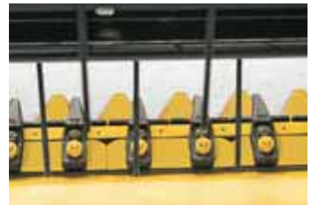
Hydraulic-driven, dual, counter-stroking sickles are belt-timed for a swift 1828-spm knife speed for fast, clean cutting.
