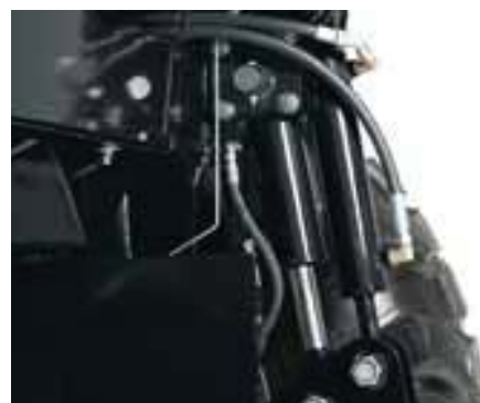
Adjustable cut height cylinders on each lift arm make it easy to return to the pre-set cutting height after each pass.
