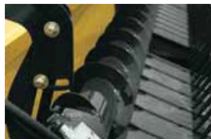
Optional feed auger is hydraulically driven on draper headers to help move extremely heavy or high-volume crops into the windrow opening.
