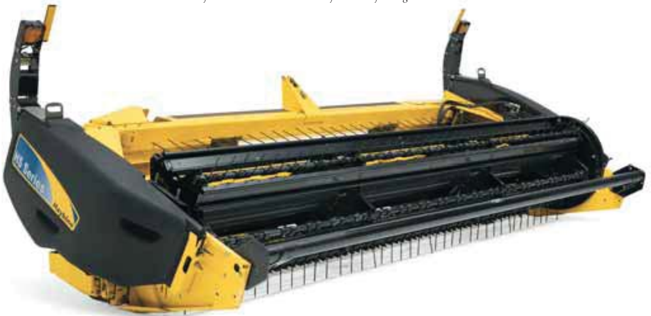
The wide opening in the header floor behind the cutterbar allows for gentle crop collection and windrow formation with the assistance of windrow forming rods.
