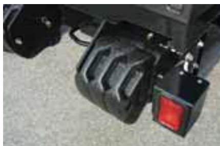
Optional rear weight bracket and weights may be installed on any H8000 model to balance heavy or wide heads.
