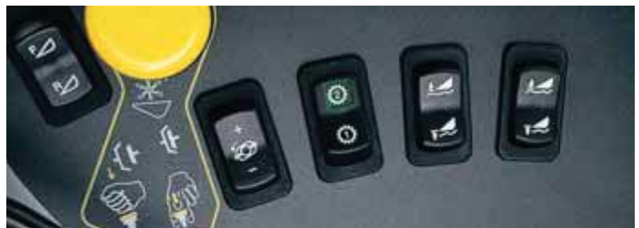
Dual switches in the H8060 and H8080 cab allow you to control the flotation of the left and right side of the header independently.
