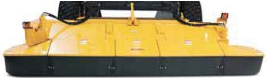
The new MowMax cutterbar is a truly modular design with independent sealed disc modules. Durability is built into the design with heavy cast rock guards, hardened alloy drive shafts, replaceable skid shoes and superior lubrication.
