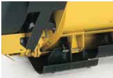
Five-position adjustable skid shoes allow you to set the cutting height quickly, without tools.
