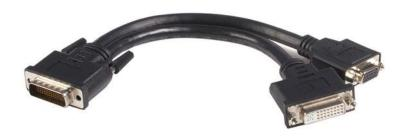
This DMS 59 to DVI and VGA Y cable allows you to break out one LFH 59 or LFH 60 (DMS 59 and DMS 60) connection on Matrox Qid, nVidia Quadro, and PNY Quadro cards into one DVI-I dual link female connector and one high density DB15 female connector, letting you to connect one VGA monitor and one DVI monitor for a cost-effective dual display solution.
