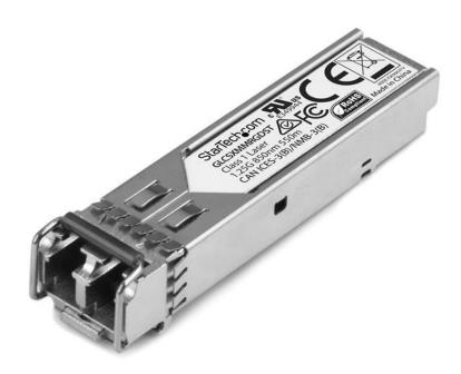
The GLCSXMMRGDST is a Cisco GLC-SX-MM-RGD compatible fiber transceiver module that has been designed, programmed and tested to work with Cisco® brand switches and routers. It delivers dependable 1 GbE connectivity over fiber cable, for 1000BASE-SX compliant networks, with a maximum distance of up to 550 m (1804 ft).
