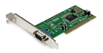
The PCI1S550 16550 Serial PCI Card can be installed in a PCI slot to add one RS232 serial port - a costeffective solution for connecting any new serial device or old legacy serial device, with data transfer rates of up to 115.2 Kbps.
