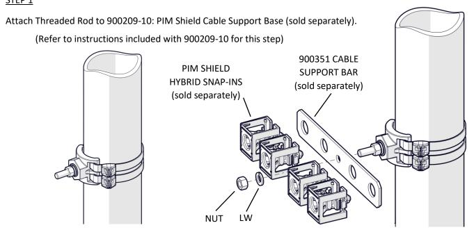
Install Cable Support Bar with hardware as shown (Torque hardware to 10 Ft-lb, ConcealFab Tool PN: 900053) (Note: Spare washers supplied with kit), then attach hybrid snap-in support(s) (sold-separately).
