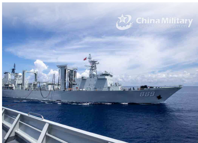
Sailors assigned to the 39th Chinese naval escort taskforce connect a fuel probe from the comprehensive supply ship Taihu (Hull 889) to their ship during a replenishment-at-sea operation in waters of the South China Sea on October 1, 2021. (eng.chinamil.com.cn/ Photo by Zhao Yang)
