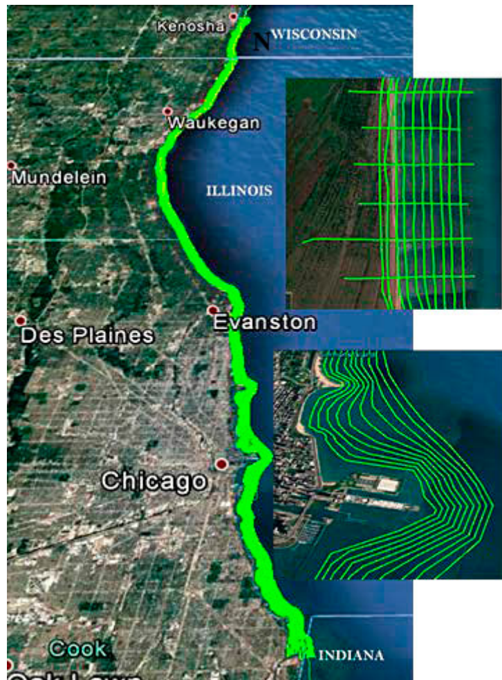
Figure 9-56. Map showing the helicopter survey lines (green) at 100 m spacing, on the southwestern Lake Michigan shore. The top inset show example of perpendicular flight lines east of Illinois Beach State Park (IBSP). The bottom inset show the flight lines ~100 m away from infrastructures and buildings in Chicago.
