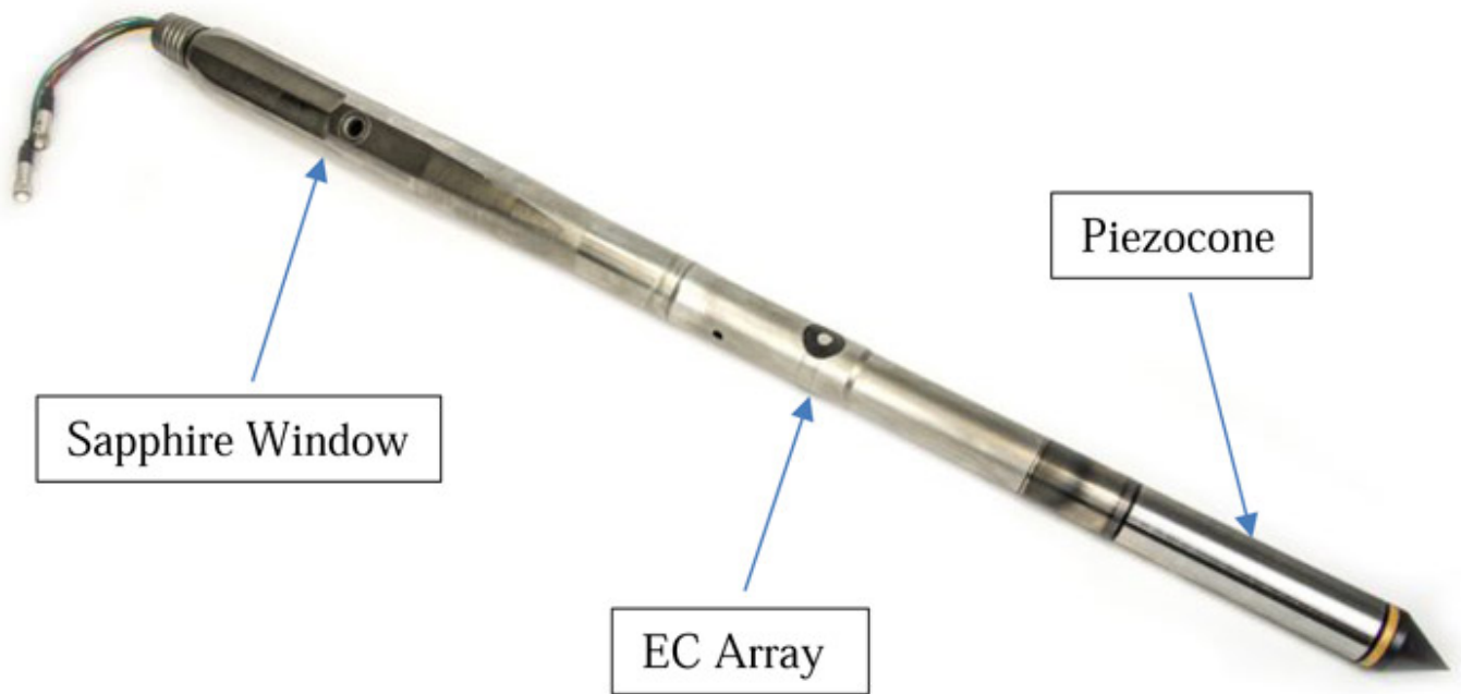
Figure 3-9. OIP probe with attached CPT cone.
