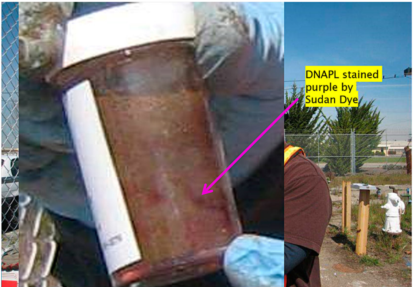
Figure 9-7. Sudan Dye staining indicating TCE DNAPL.
