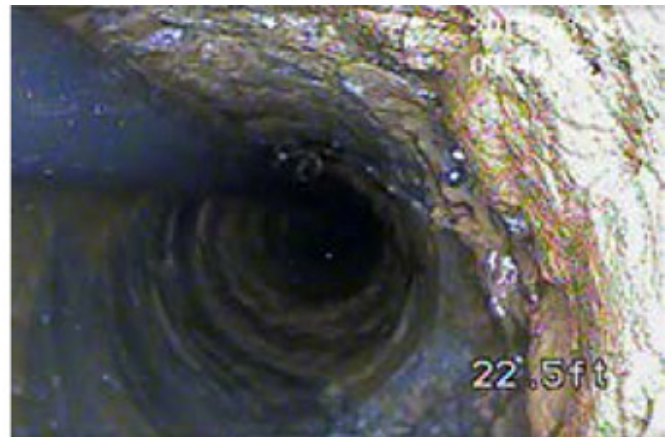
Downhole view of borehole wall. Note groundwater flow on right side of image.
