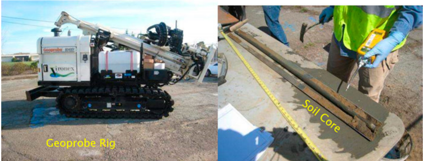
Figure 9-6. Soil core collection with Geoprobe DT8040.
