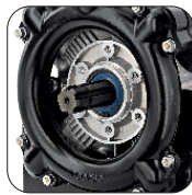
C/C Version 1 3/8" 6 Splined Thru Shaft.
