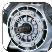
C/C Version 1 3/8" 6 Splined Thru Shaft.
