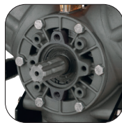
C/C Version 1 3/8" 6 Splined Thru Shaft.
