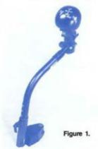
fall away when struck vertically during a crash event. On the other hand, the design has demonstrated the strength to sustain emergency flight control (hydraulics off) loads in the longitudinal and lateral directions.
