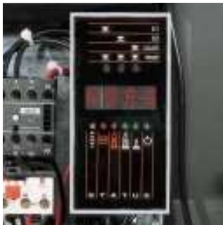
Example of "STATUS PANEL"
