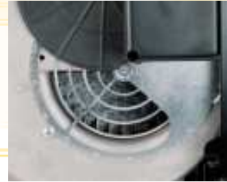
Air damper completely open
