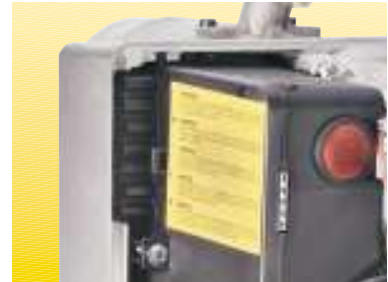
Appliance fitted with an ignition transformer
