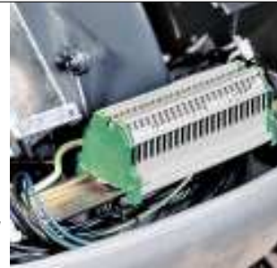
Example of the terminal board for electrical connections for the RS 68-120-160/M BLU models
