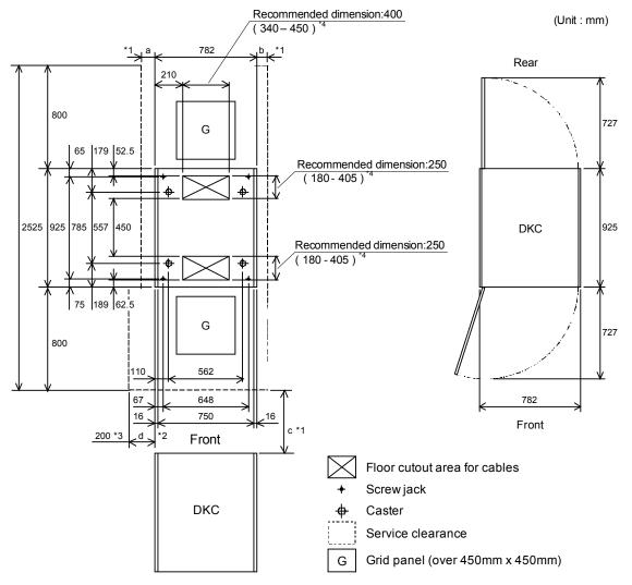
Figure 4.3 DKC Service Clearance and Floor Cutout
