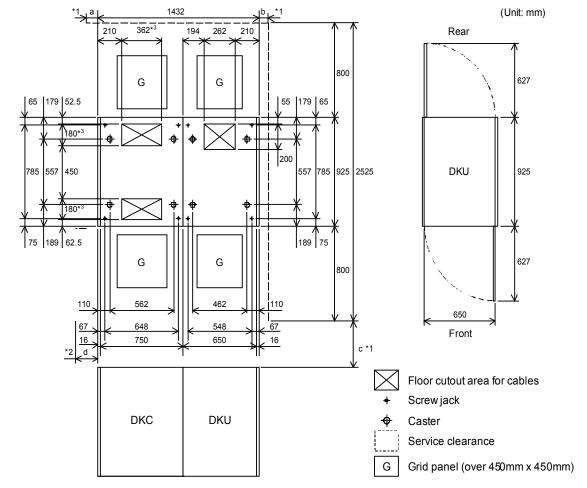
Figure 4.4 Service Clearance and Floor Cutouts for Two Frames
