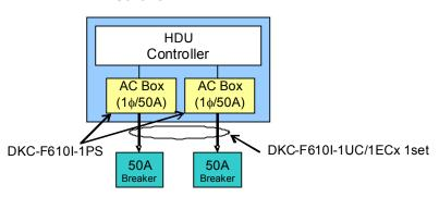
Figure 4.9 Single-Phase AC Input Power (DKC)
