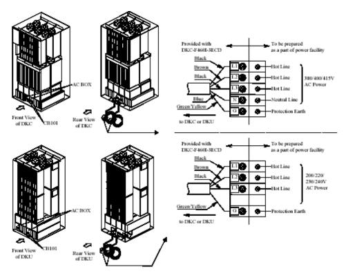
Figure 4.7 Three-Phase 30-Amp Model for Europe
