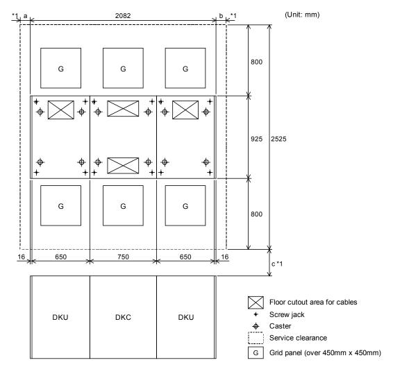
Figure 4.5 Service Clearance and Floor Cutouts for Three Frames
