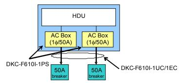
Figure 4.10 Single-Phase AC Input Power (DKU)
