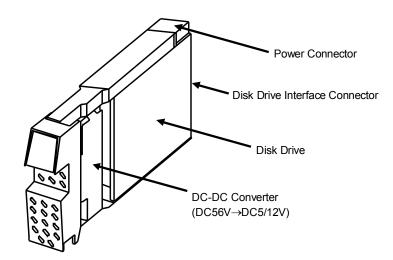
In the canister that is mounted with the HDD above, the DC-DC converter, which converts 56V DC to 5V and 12V DC used by the HDD, is installed.
