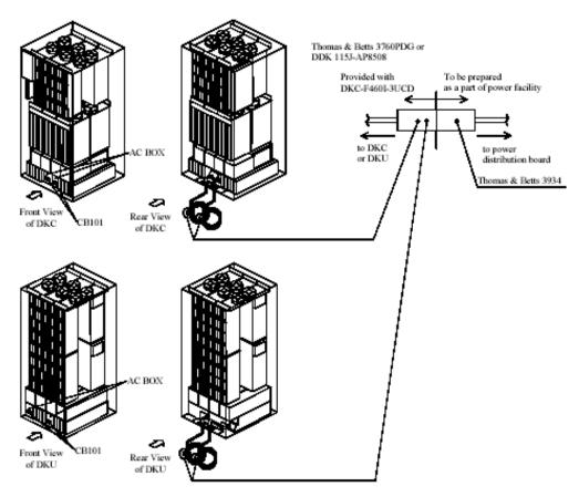
Figure 4.8 Three-Phase 30-Amp Model for USA
