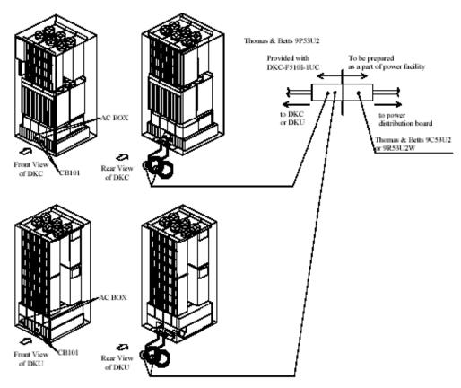
Figure 4.12 Single-Phase 50-Amp Model for USA
