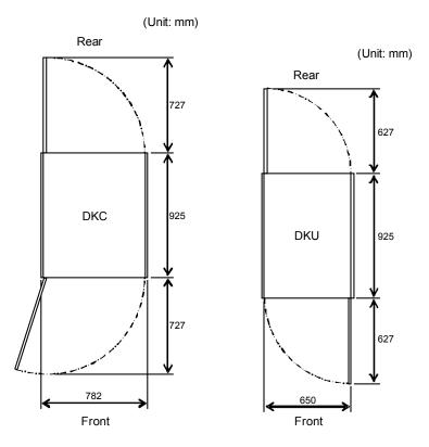
Figure 4.2 DKC and DKU Physical Dimensions for the Universal Storage Platform V
