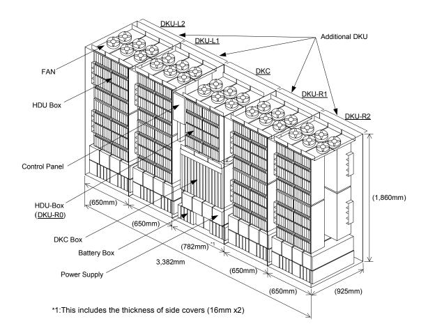
Figure 4.1 Physical Overview of Universal Storage Platform V
