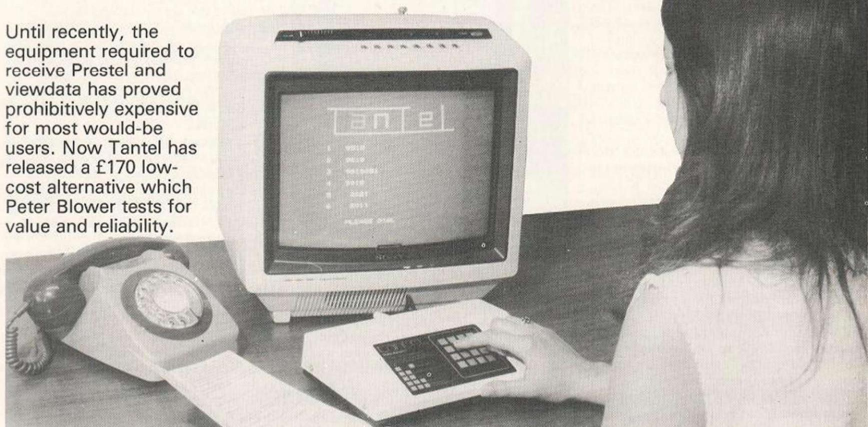
THE DEVICE tested contains an issue 2 board carrying Version 2.2 EPROM. The whole board is small, but heavy for its size — 243mm. by 165mm. by 58mm. weight: 2kg. — and has three leads connecting it to the outside world.
