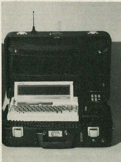
CELLULAR TELEPHONE, MODEM, computer and software make up a complete portable office, usable in a car or on the beach.
