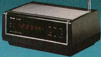
Most Accurate Clock uses NBS atomic clock signal to keep "perfect" UTS time.
