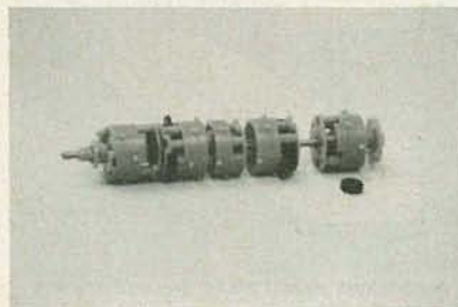
FIG. 5—THE PLANETARY GEARING SYSTEM. Don't throw this out! You'll need six \frac{3}{8} -inch gears from the system.
