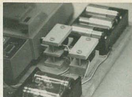
FIG. 10—THE MOTOR-MOUNTING BLOCKS on the right side of the Armatron .
