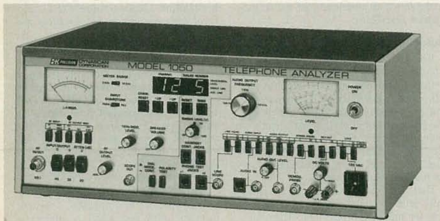
FIG. 3—THE B + K 1050 telephone analyzer contains many instruments and features required to adequately service a cordless telephone.
