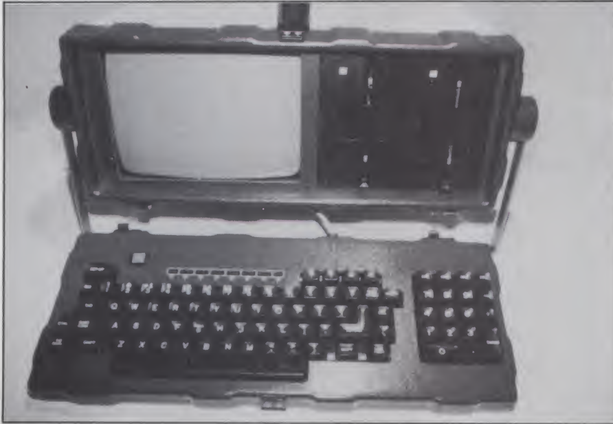
In its standard configuration, the M6000P has two 376K 5¼-inch disk drives. All units come with a detachable VT100-style keyboard.
