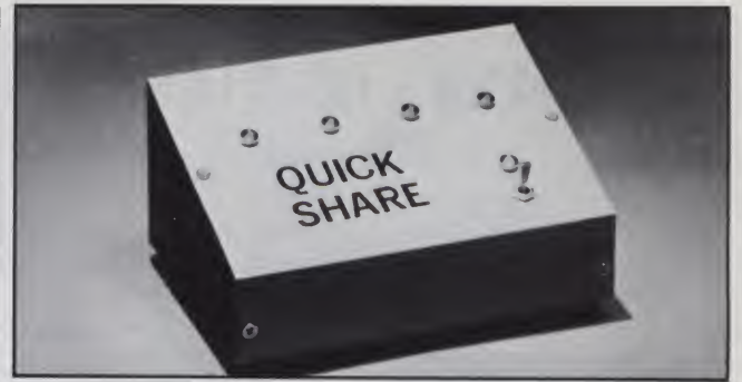
Quick Share, from Wolsten's Computer Devices, allows four Atari 400, 800, or 1200 computers to share up to four disk drives, one printer and one software program.
