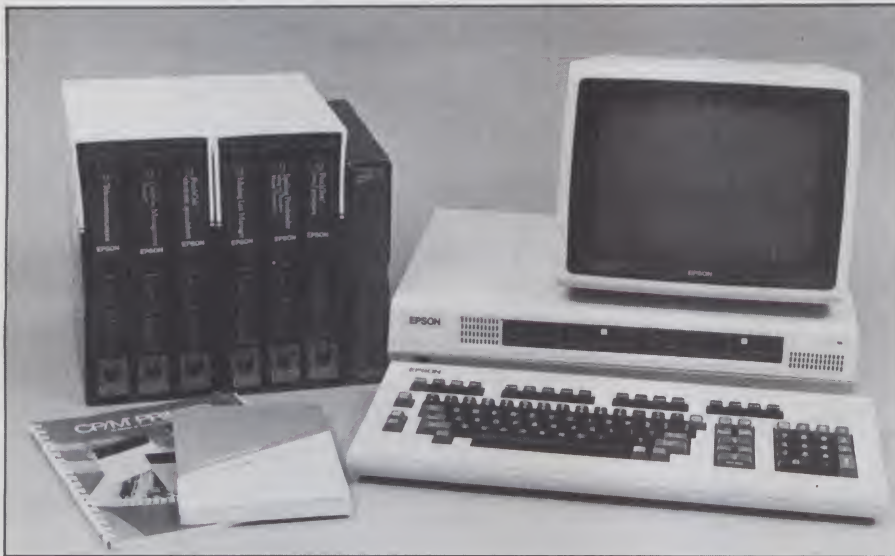
The Epson QX-10 and software documentation. The six-volume set of Peachtree software will be Epson's first applications software release. Also shown is the CP+ manual, CP/M Primer and the Microsoft Basic manual, part of the documentation supplied with the CP/M-based QX-10 system. (Photos by Jim Hansen.)
