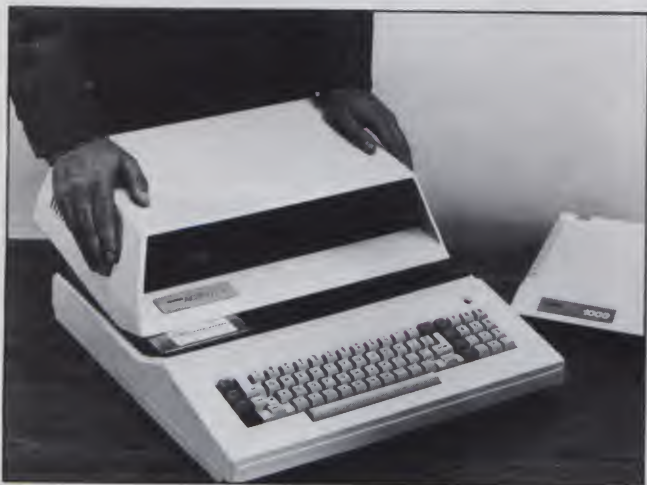
The ACE 1100, Franklin Computer Corporation, is an add-on disk drive unit for the Franklin ACE 1000.
