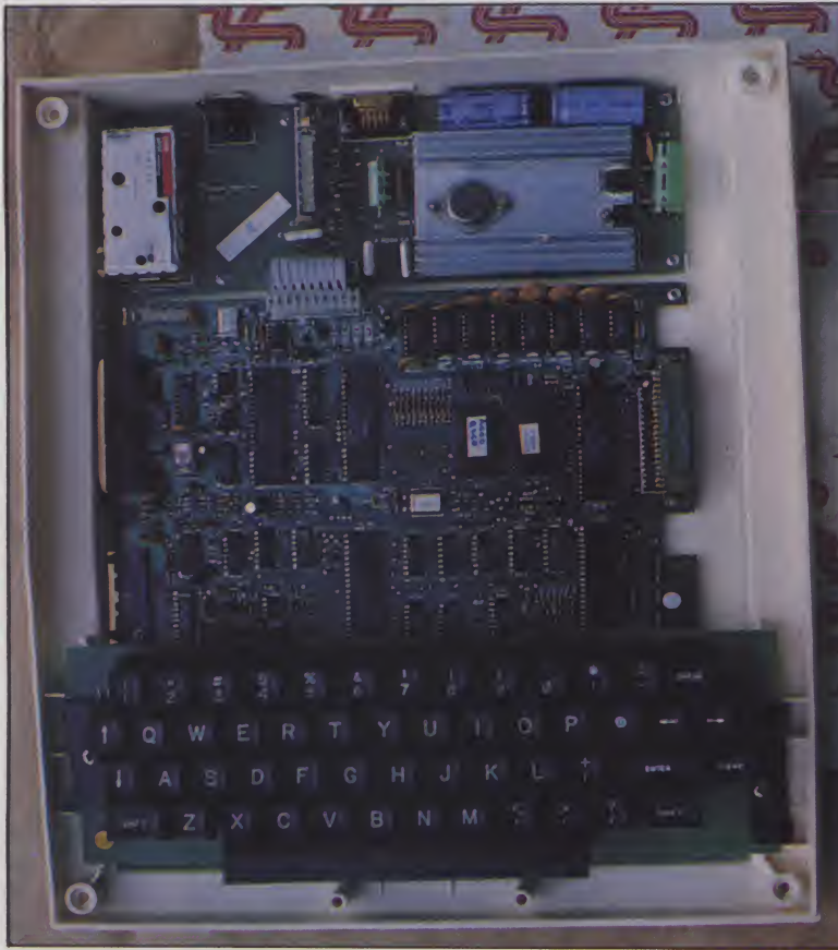
The Dragon's keyboard and components are of high quality—and similar to those of Tandy machines. The only difference immediately apparent is the provision of a parallel printer output port rather than the RS-232 port.
