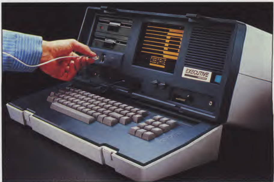
The Executive is slightly bigger than the Osborne 1, but the screen is larger, too. The seven-inch amber screen presents a clear, sharp display.
