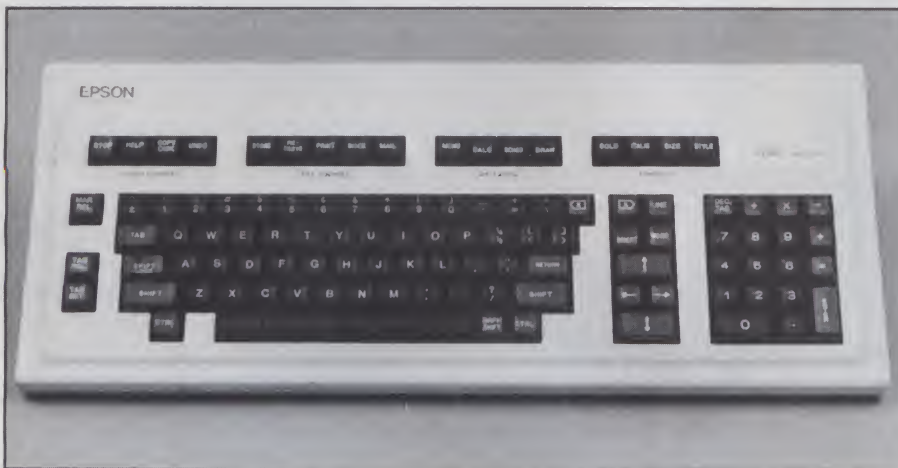
The HASCI keyboard used with Valdocs on the QX-10. Notice the Selectric-like keyboard layout in the typing section. The editing cluster and numeric pad are to the right. Above the typing section are the Valdocs function keys. The Valdocs QX-10 can also run TPM (a fast CP/M look-alike) or CP/M 2.2.
